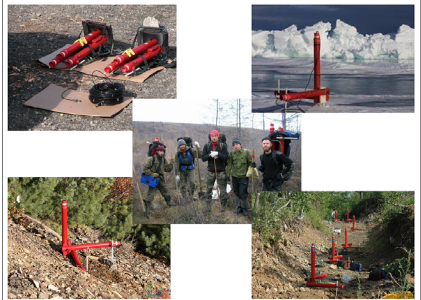
Figure 4: Centre: crew ready to transport tripods to site. Clockwise from top left: tripods with three sensors folded for transport by backpack; installation for an AMT survey site on a frozen lake; installed at close spacing on level ground; installed on a steep slope.
