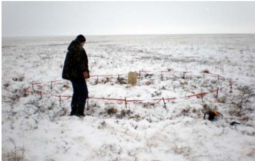
Preparation of CS grounding (grounded cable).
