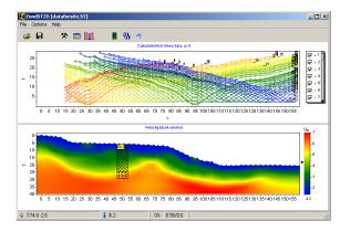
ZondST2D is designed for 2D data processing and interpretation of seismic tomography by method of refracted waives. There are several options:
